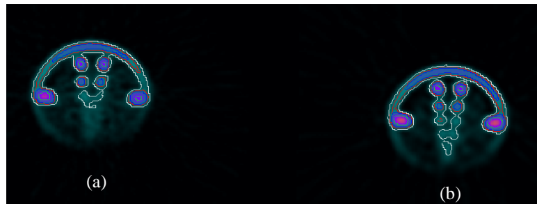
Fig.5: (a) and (b) Show the hot region images (a) without and (b) with copper 0.127 mm material filter
